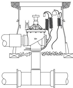
**Heavy Duty 3" Remote Control Valve Globe Installation**
