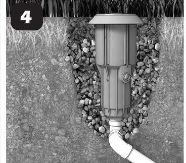
**4** Fill hole with gravel covered by a layer of soil.
